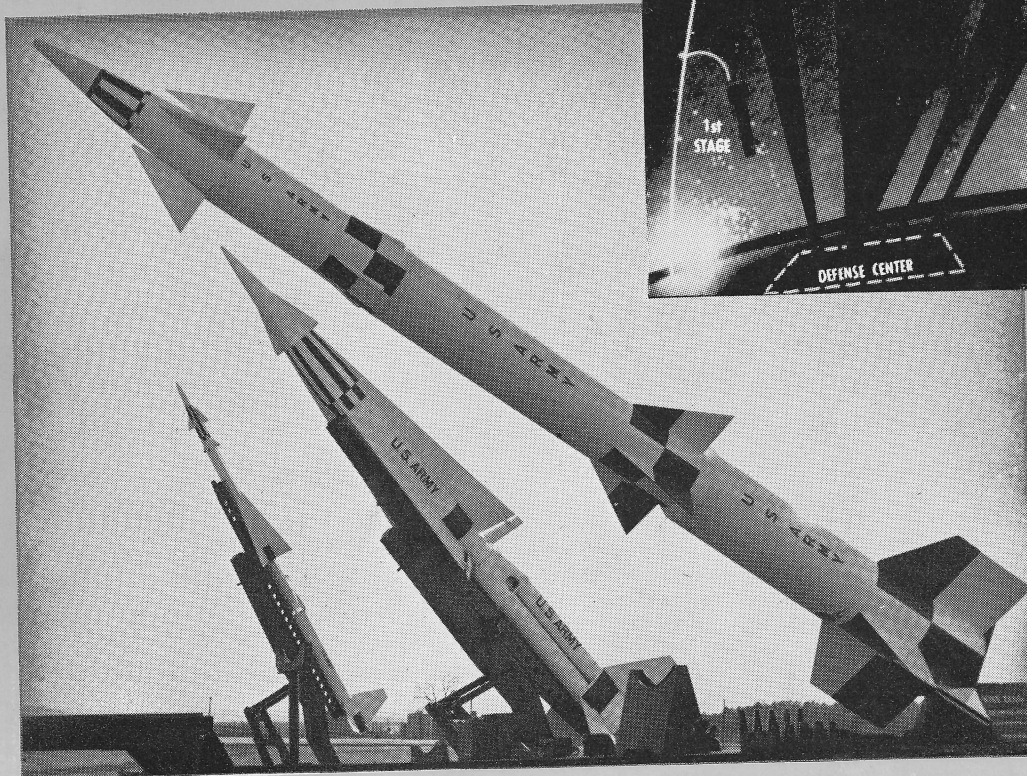
Above, graphic sketch shows Nike Zeus reaction time. At left, the Nike family poses for a portrait: from left to right, Ajax, Hercules, Zeus.
